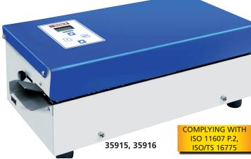
• 35915 D-600 ROTARY HEAT SEALER - without printer • 35916 D-700 ROTARY HEAT SEALER - with printer With validation system complying with ISO 11607 P.2 rule. GIMA 600 and GIMA 700 have been designed to continuously monitor, during the whole sealing phase, all critical process parameters: Temperature, Speed, Pressure. They guarantee sealing in full respect of EN 868-5 / ISO 11607 P.2 rules, provide real-time monitoring of working temperature, applied force
